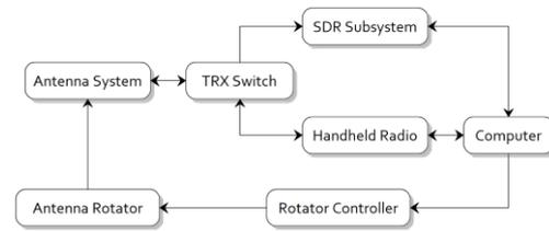
Fig. 7. Block diagram of the ARSS kit.
