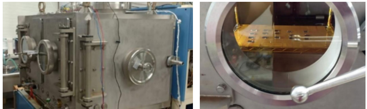
Maya-2 Thermal Vacuum Test
