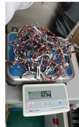
Weighing of all wire harnesses for mass budget calculations
