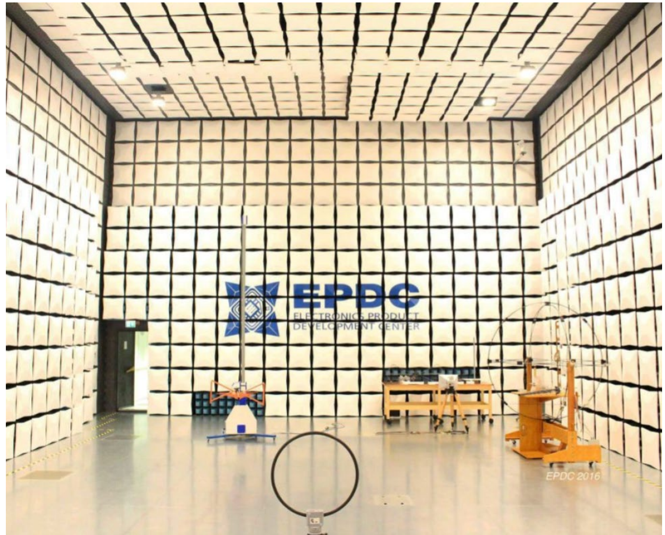
Semi Anechoic Chamber in EPDC Photo courtesy of EPDC
