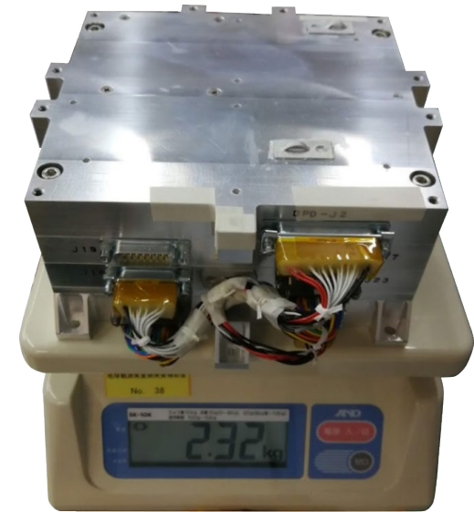
Mass measurement of Diwata-2 Satellite Central Unit (SCU)
