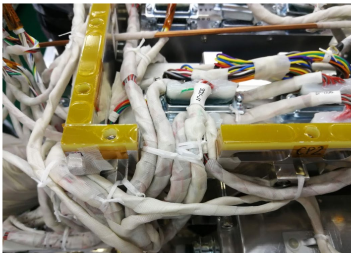
Integration of wire harness during assembly phase
