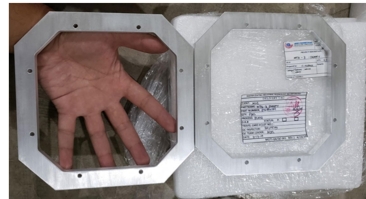
Sample fabricated dummy masses
