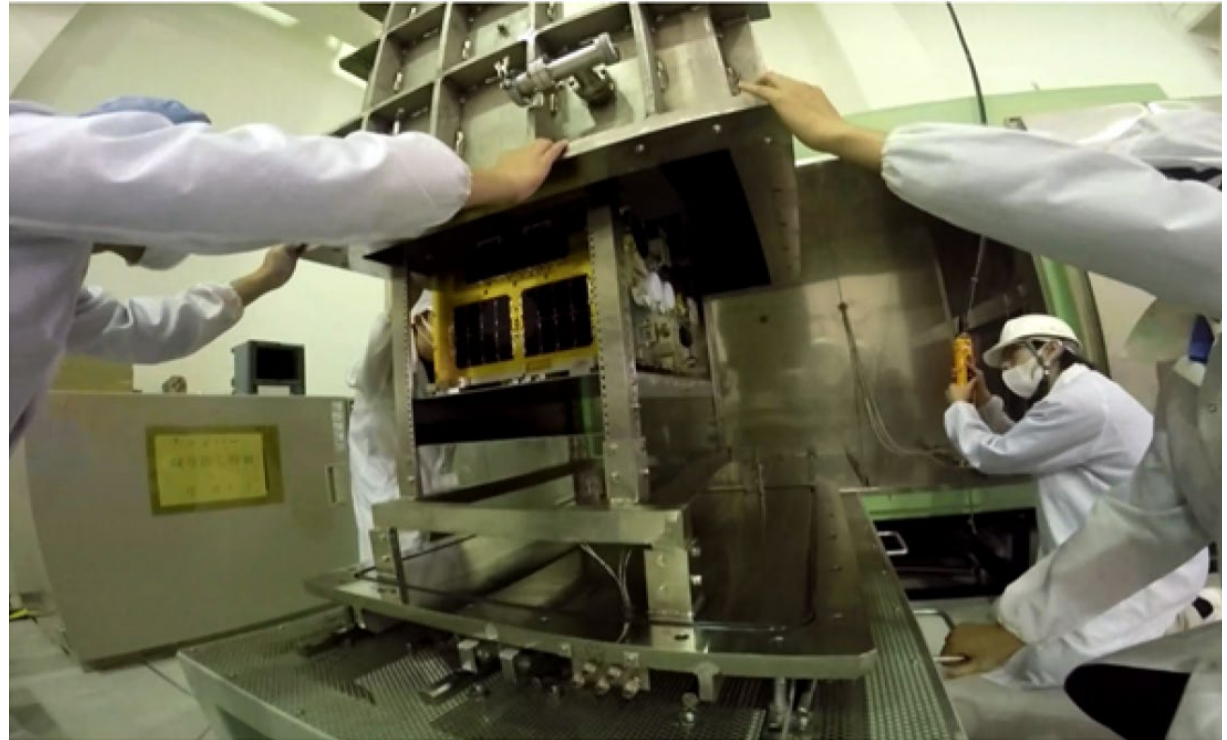
Diwata-1 before undergoing off-gas testing at JAXA's facility in Tsukuba, Japan
